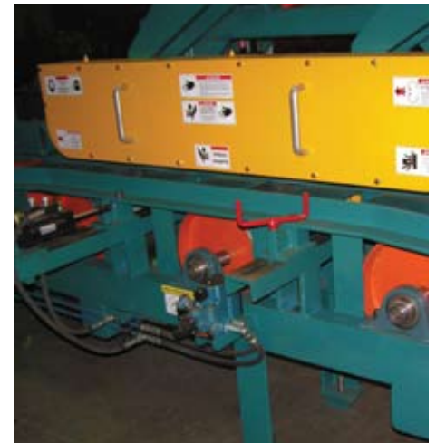
The powered holddown assembly features 3 x 16" diameter knurled and chromed rolls. Dual hydraulic cylinders allow remote positioning and tensioning of the powered holddown.
