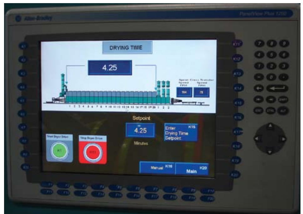
The controls system on the TRVP dryer makes it easy to set the drying "recipes" to maximize throughput.
