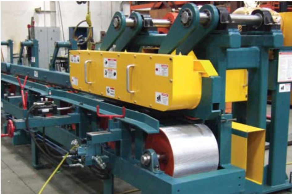
The powered holddown assembly features 3 x 16" diameter knurled and chromed rolls. Dual hydraulic cylinders allow remote positioning and tensioning of the powered holddown.
